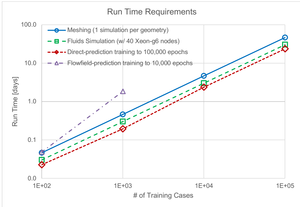
Figure 17. Meshing, fluids simulation, and model training run time requirements vs. total number of training cases.
