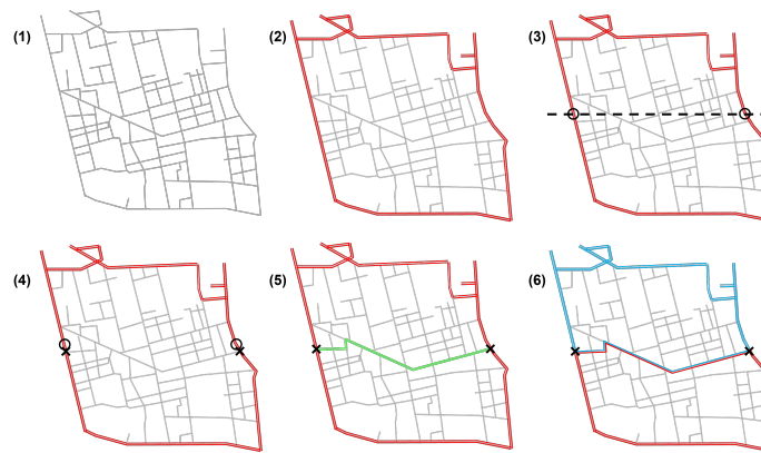
Figure 6: (1) The initial street network; (2) The perimeter of the street network identified through Algorithm A1; (3) A horizontal divider and the pierce points where it crosses the perimeter; (4) The pierce points and the nearest perimeter nodes; (5) The shortest path on the road network between the two perimeter nodes; (6) The perimeters of the two regions produced from the proposed cut
