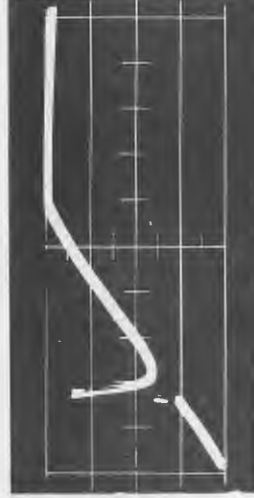
V416, Pin 3 120 Volts Peak to Peak 20 \mu s/cm
