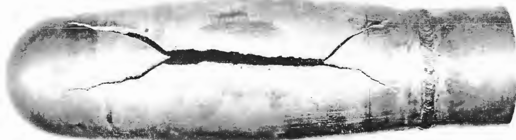
Fig. 5 Result of Cold Hydrostatic Burst Test
