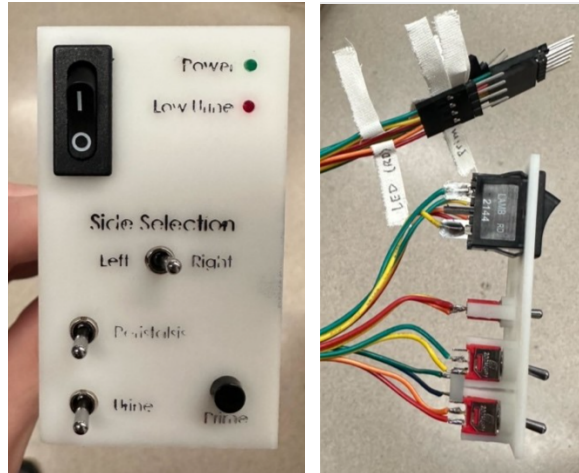
Figure 178: Prototype of the physical control interface to control peristalsis and urine leakage
