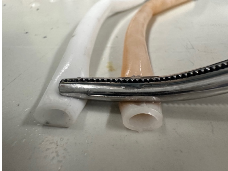
Figure 31: Comparison of PVA ureter samples. The chosen ureter, right, includes nylon mesh
