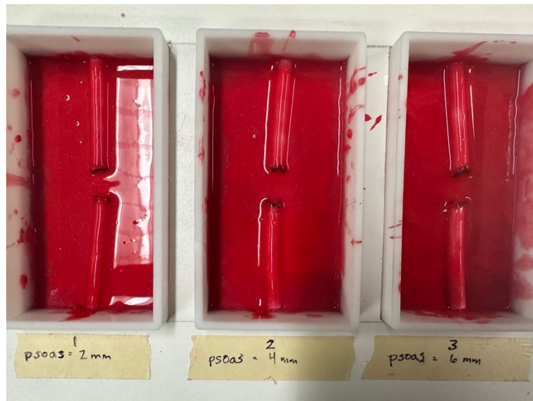
Figure 27: Prototyping multi-layer pucks with embedded, injured ureters
