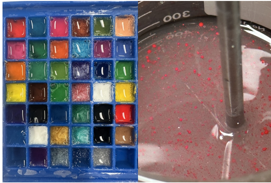
Figure 24: Sample color palette of PVA (left) and PVA being mixed with simulated blood dispersion (right)
