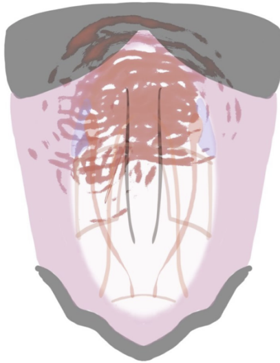
Figure 7: Outline of silicone Abdominal Sock (pink) in relation to the rigid Base Cradle (gray)
