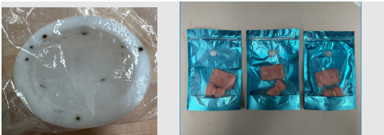
Figure 29: Potential bacterial/mold growth on PVA (left) and testing storage solutions (right).
