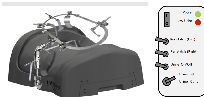
Figure 6: Mockup of Base Cradle and Bookwalter retractor (Left) and a mockup of the physical control interface to control peristalsis and urine leakage (Right)
