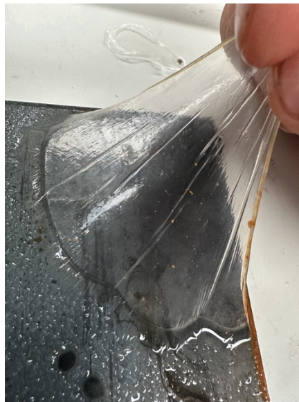
Figure25: Example of thin membrane of PVA achieved through spray application
