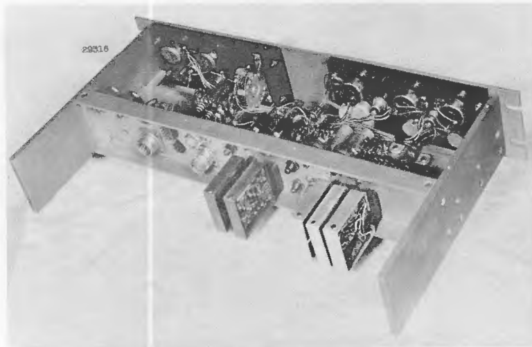
Fig. 6 - The Retrace Insertion Unit chassis showing the subminiature plug-in circuit packages
