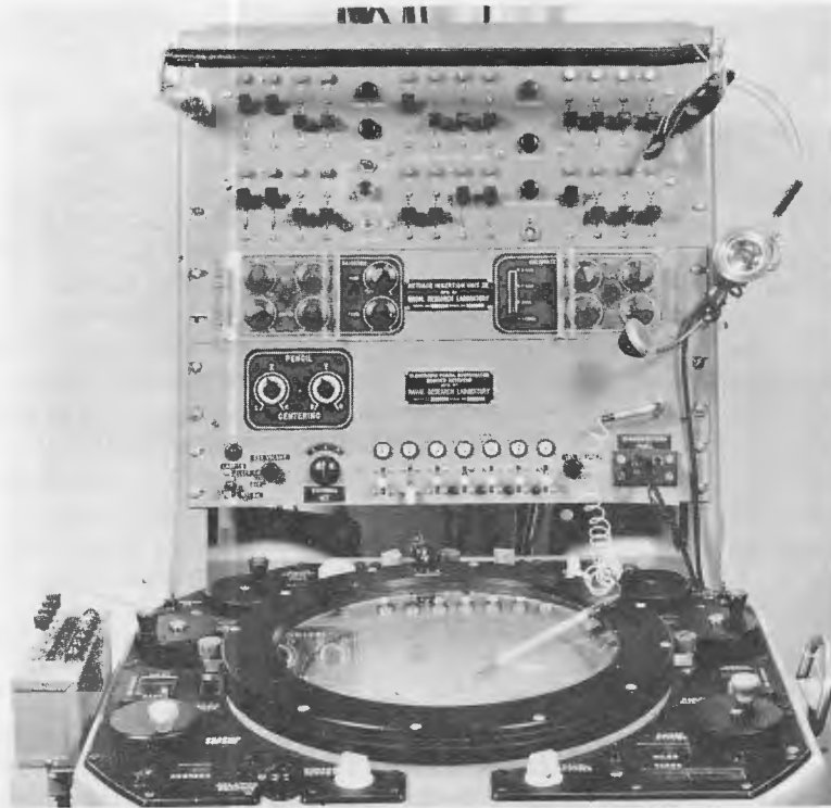
Fig. 2 - A typical EDS Detector or Tracker Console showing the Store Control Panel, the Retrace Insertion Unit, the Electronic Pencil Coordinator, the Communication Panel, and the EPC conducting-glass head in place over the SPA-8A PPI. The push-button box on the left of the PPI is associated with the Velocity Derivation feature for aided tracking.
