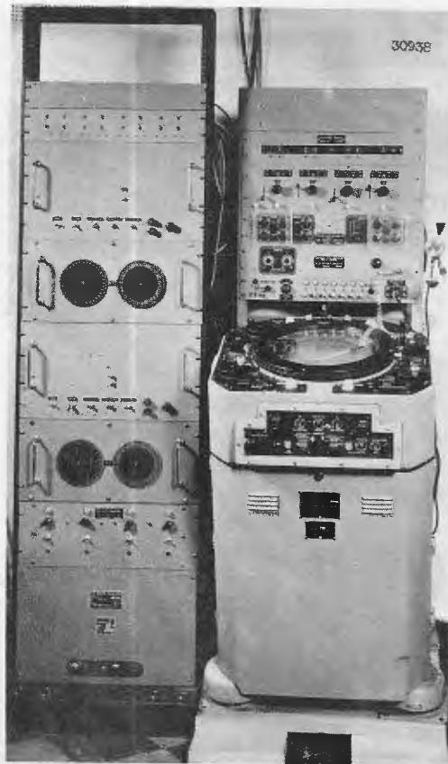
Fig. 19 - The Target Designation Console and coordinate converter rack including equipment for designating to two fire control director radars.
