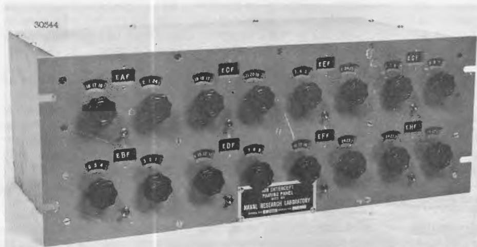
Fig. 28 - The Air Intercept Pairing Panel with facilities for 16 targets or 8 intercepts
