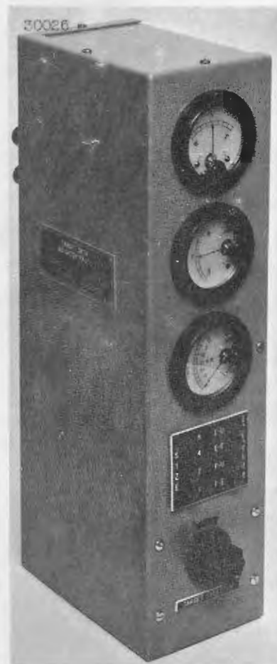
Fig. 16 - The Target Data Indicator Panel Permitting plan position, height, size, and identity to be selected by track number.
