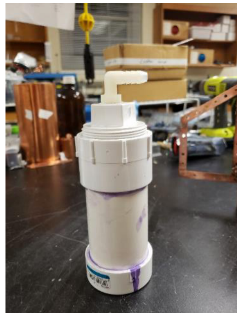
Figure S3.26. The Battery and Timer Compartment Were Made with PVC Cleanout Adaptor with Plug, PVC Socket Cap, and a 90-Degree Hose Barb.
