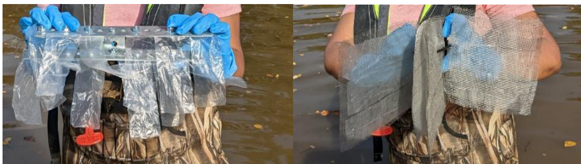
Figure 5.4. Field Deployment of Optimized Passive Samplers (0.7 mil PE) in Exposed (Left) and Mesh-enclosed (Right) Configurations for Short Term Measurements of Surface Water PCB Concentrations.
