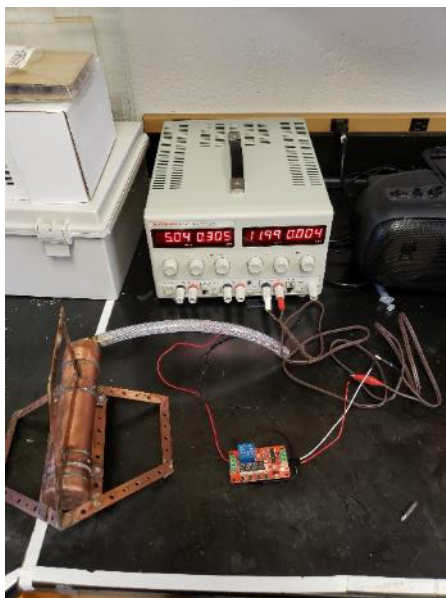
Figure S3.31. Power Bank Displaying the Current Required to Run the Vibrating ~4mA
