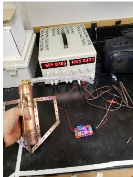
Figure S3.32. Power Bank displaying the Current Required to Run the Vibrating ~400 mA
