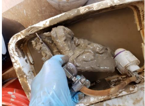
Figure S3.28. During the Experiment the Clay-like Mud Clumped onto the Sampler.
