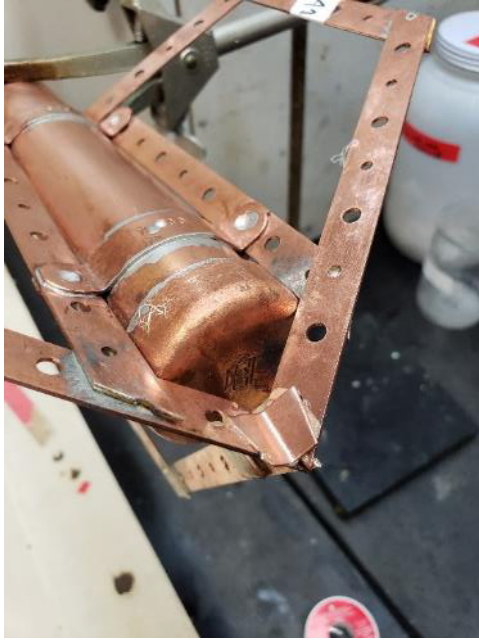
Figure S3.23. A Scrap Piece of Copper Was Bent to Conform to the Angle of the Wings.
