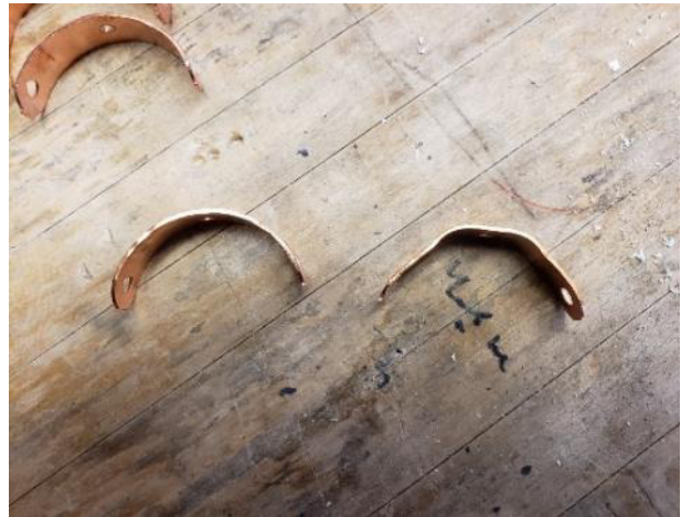
Figure S3.8. A Side-by-side Comparison of the Strap Before (Left) and After (Right) Shaping them.
