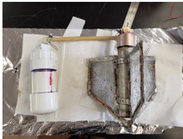
Figure S3.29. The Vibrating Sampler After the First Experiment in Mud.
