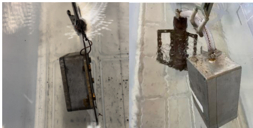
Figure 5.3. Vibrating Passive Sampling Platforms, P1-14G (left) and P2-110G (Right), With PRC Loaded PEs Suspended in Outer Reservoir of DI Water to Track Fractional Approach to Equilibrium in Low Frequency and High Frequency Modes.
