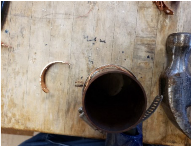
Figure S3.7. The Pipe Clamp Was Placed on Top of the Strap.
