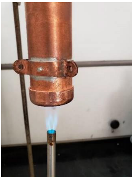
Figure S3.13. A 1 1/2 in. ID End Cap Is Used to Seal on End of the Sampler.
