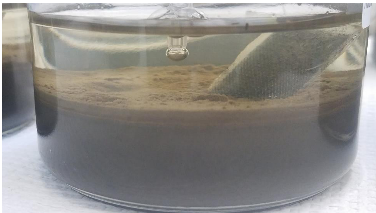
Figure S7.1. Sediment Microcosm Displaying a Sheet-ps Sampler Inserted Across the Sediment-water Interface.
