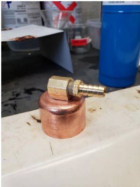
Figure S3.25. The Cap Was Made Using a 1/2 in Copper End Cap, Brass Hose Barb, and a Brass Street Elbow.
