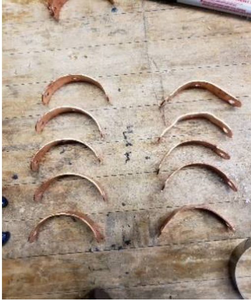
Figure S3.9. Before and After Shaping the Strap to the Body of the Vibrating Sampler.
