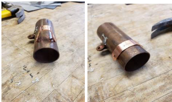
Figure S3.4. The Final Rough Shape of the Strap After Shaping it with a Hammer.
