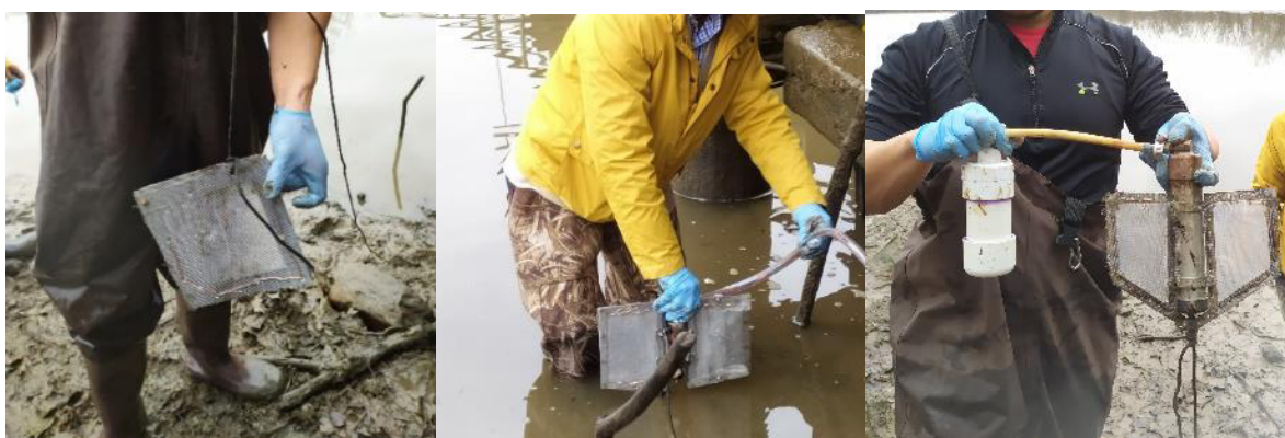
Figure 3.2c. Deployment of Static (Left) and Vibrating Passive Samplers P2-125G (Middle) and P2-110G (Right) at Kingman Lake, Washington DC on 10 December, 2019.
