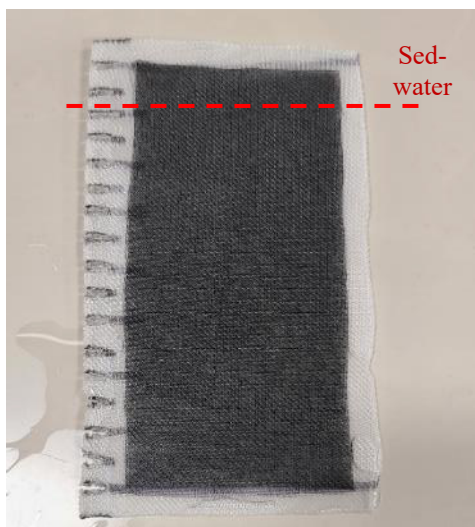
Figure 8.2. Passive Sampler Synthesized for Aqueous Spatial MeHg Profiling within Sediment Microcosm Experiment.
