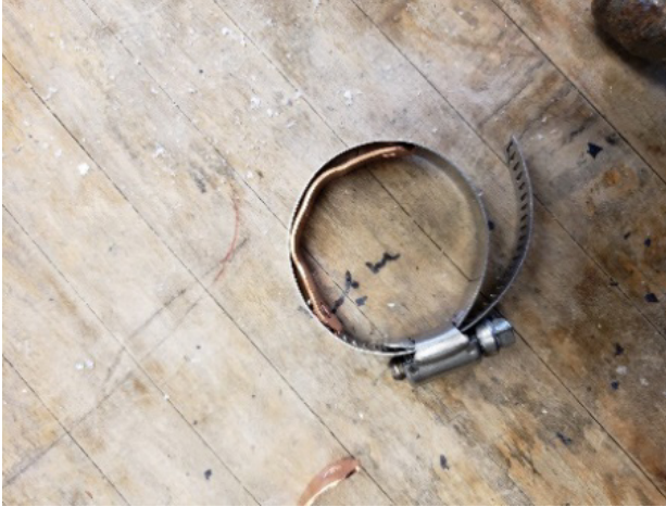
Figure S3.5. To Shape the Strap into the Final Form of the Vibrating Body a Pipe Clamp Was Used.
