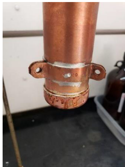
Figure S3.14. The End Result of Soldering the End Cap to the Sampler.
