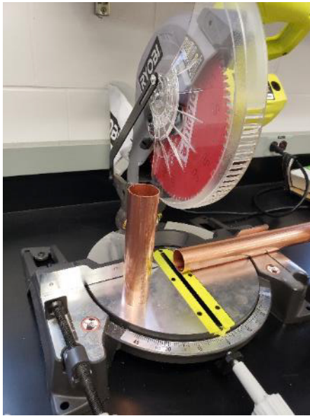
Figure S3.1. Miter Saw was Used to Cut the 1 ½ in. ID Copper Pipe to 7.25 in.
