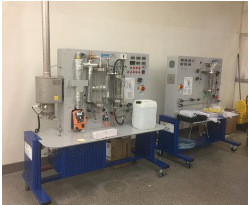
Figure 1: Steam-turbine plant in EN4-125 @ CSULB
