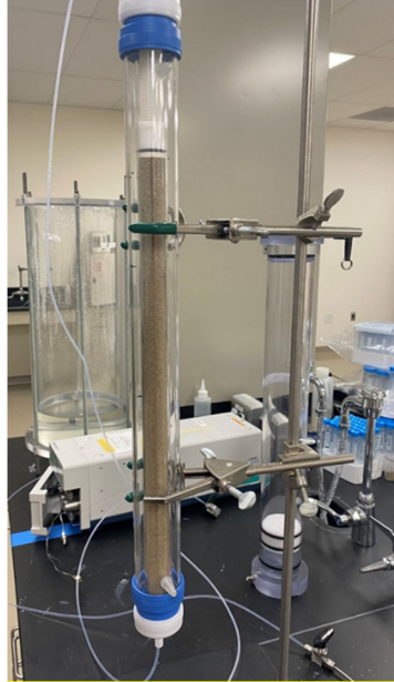
Figure 4: Experimental setup for 1-D flow experiments. A homogeneous sand pack of either US Silica OK-75 sand or C2 horizon field-obtained sand was used.
