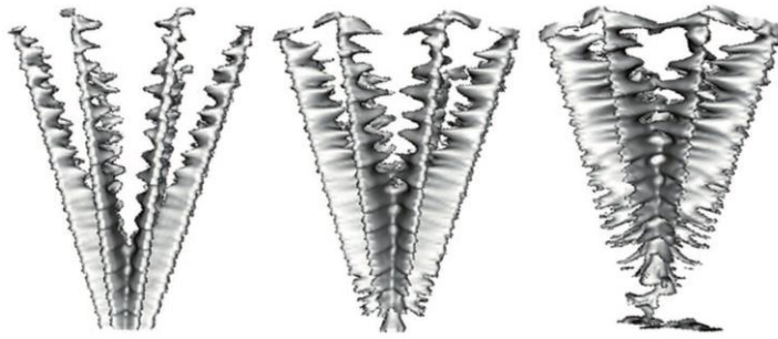
Fig. 3 Above, simulations of the zippered implosion of a conical array made by the 3D MHD Gorgon codes. Right: Soft X-ray emission from the conical array compared to a cylindrical array, demonstrating that the X-ray emission is extended in time
