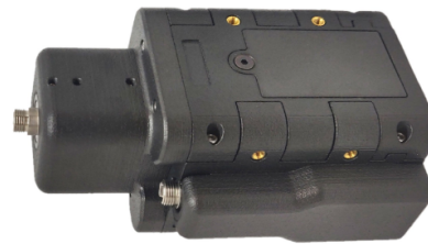
FIG. 13. PICAS system. The push beam couples in to the central fiber jack the rear, and the 2D MOT beams couple in to the other two fiber inputs (one pictured). This system contains permanent magnets within and optics used to produce the 2D MOT beam. When mounted, it fully encloses the 2D MOT cell.
