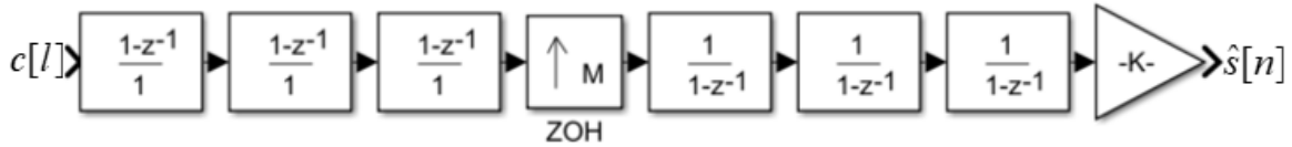
Figure 28. CIC cubic spline interpolator using the Zero-Order Hold up-sampler
