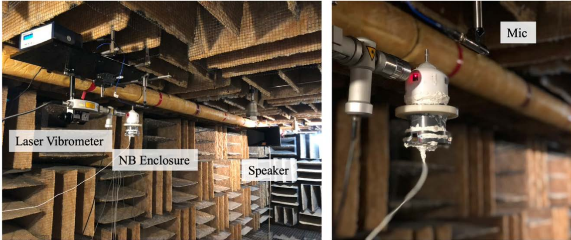
Figure 24. Enclosure vibrational response experimental setup (laser vibrometer)
