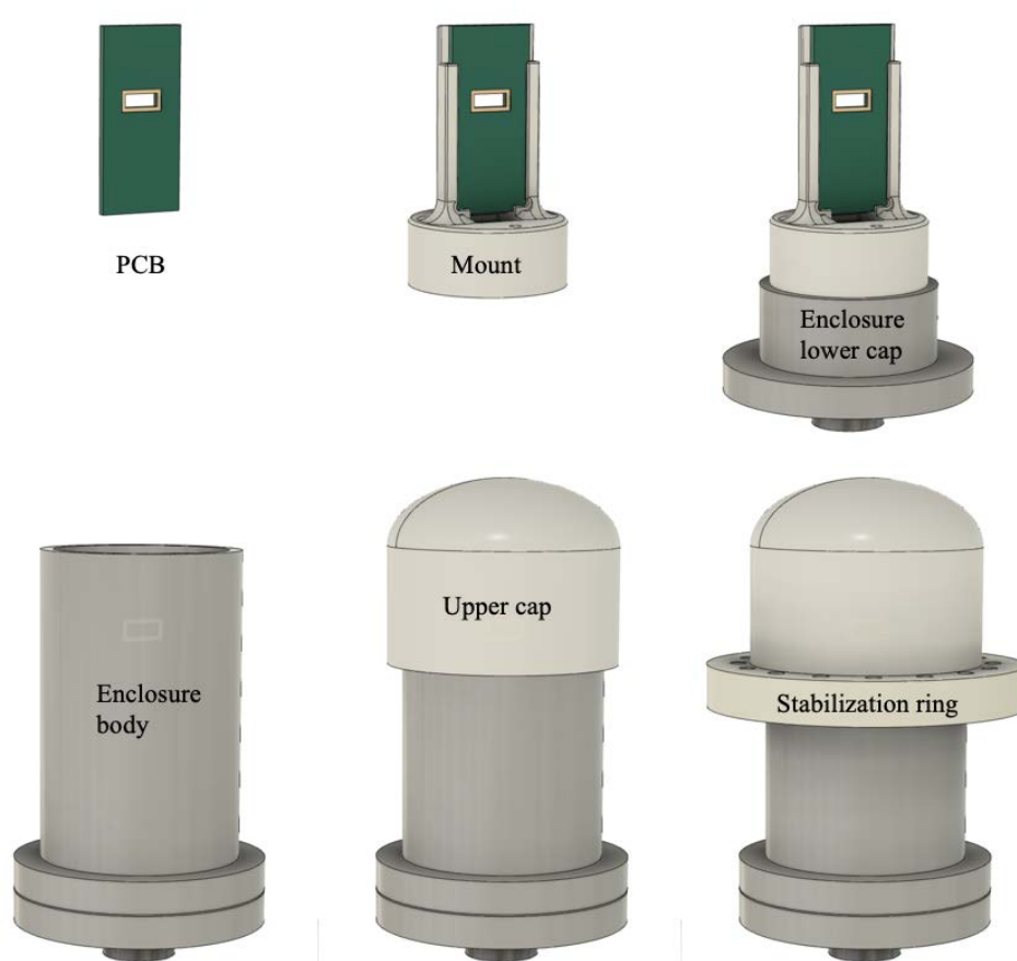
Top row, left to right: PCB and sensor (white cutout); PCB in 3D printed mount; 3D printed mount attached to NB enclosure removable end cap with vent plug. Bottom row, left to right: Removable cap in cylindrical tube (gray); permanently cemented endcap (white); enclosure with stabilizing ring.
