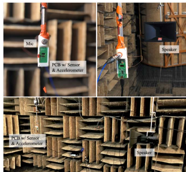
Top left: Front view of the sensor and microphone. Top right: Rear view of the sensor and microphone facing the speaker. Bottom: Wide angle view of both the sensor and the speaker
