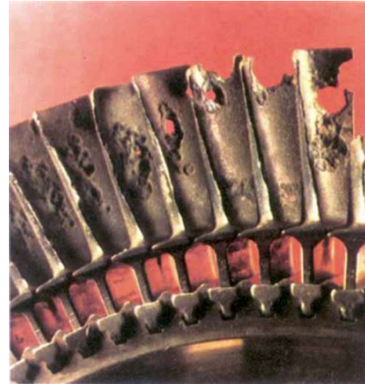
Hot corrosion, marine
