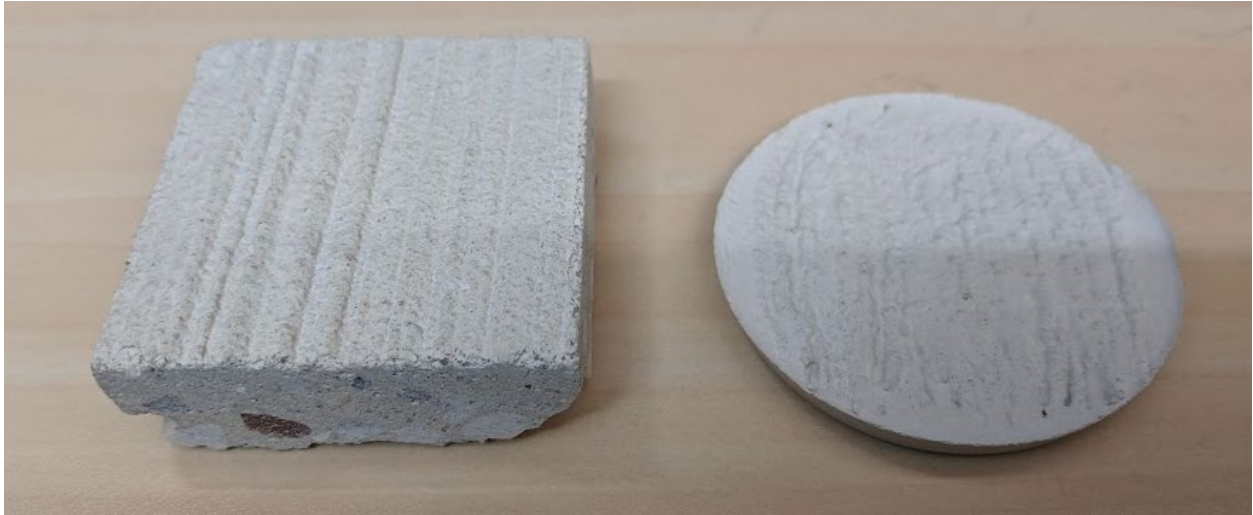
Figure 3. (Left) Thick concrete coupon and (right) 1/8 in. thick calcium sulfoaluminate (CSA) quick-set coupon.
