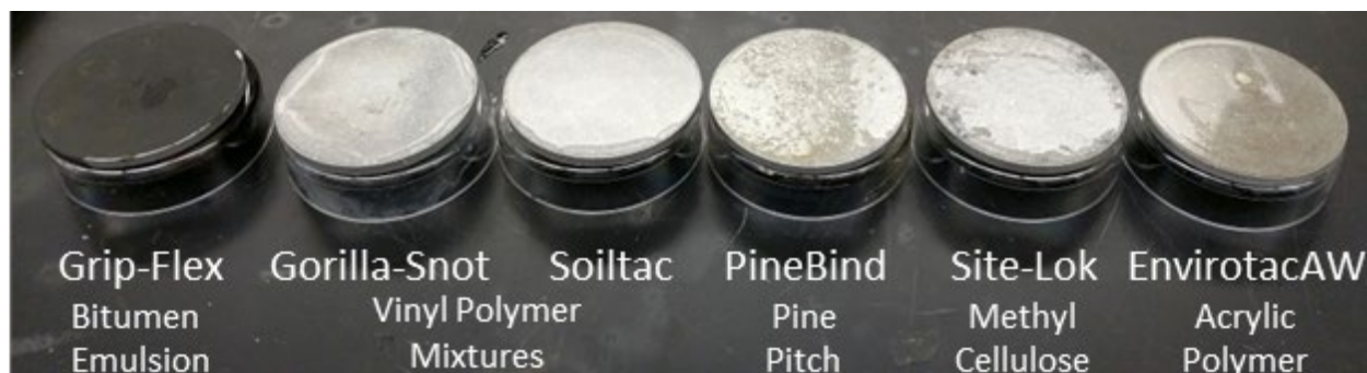
Figure 5. Application of different barrier decontaminant technologies (1 mL each) to 2 in. aluminum coupons.
