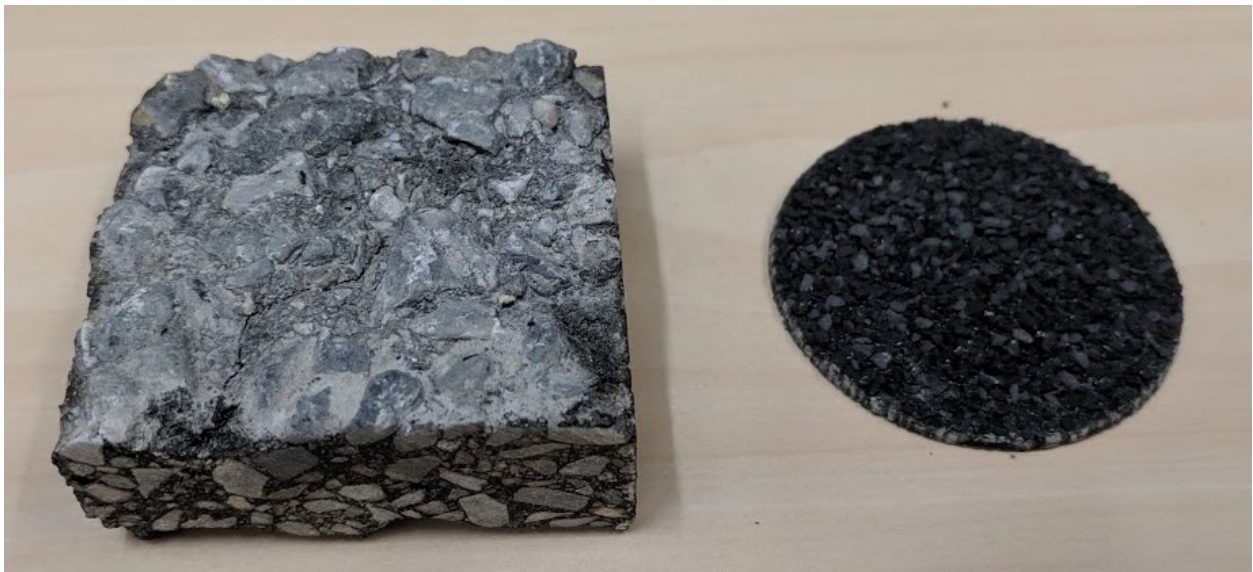
Figure 4. (Left) Thick asphalt sample from local roadway and (right) asphalt shingle coupon.
