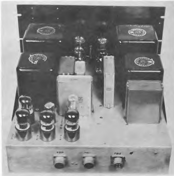
Fig. 17 - Power supply 3 and 4
