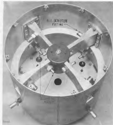
Fig. 4(c) - S-band antenna (internal, cabling removed)
