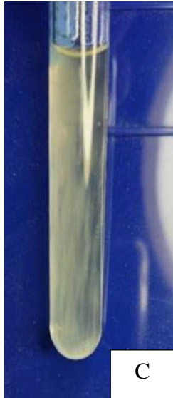
Figure 2A: Flocculent growth just below the surface of the media indicating possible aerobic and aerotolerant microbes.
