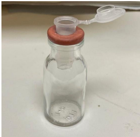
Figure 2.2: Bacterial leakage apparatus without experimental tooth.
