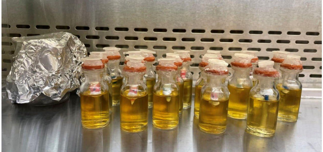
Figure 2.3: Bacterial leakage apparatus sealed with silicone.
