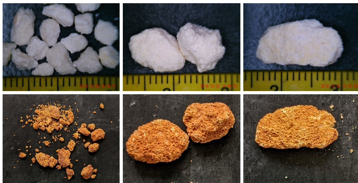
Figure 4.13. Time zero (top row) and end of experiment (bottom row) photographs for particles of IMX-101 of different sizes, small (rep a) on the left, medium (rep a) in the middle and large (rep c) on the right. Ruler division equals 1 mm. All except small particles at the end of experiment are shown at the same scale.
