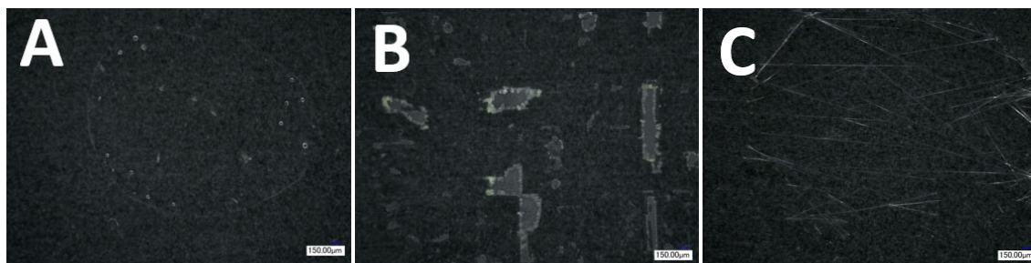
Figure 3.2. Microscope images of DNAN (A), NTO (B), and NQ (C) crystals that formed upon evaporation of 0.5 mL of 1 g L -1 DNAN (in acetonitrile), NTO (in acetonitrile), and NQ (aqueous) solutions.
