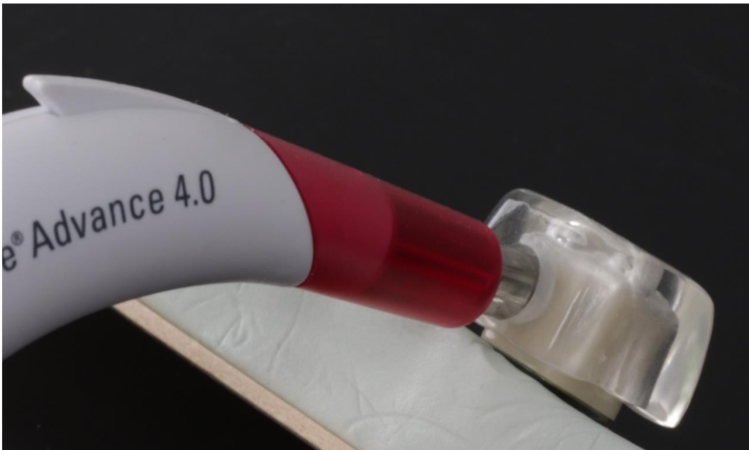
Figure 2: Clear Acrylic jig for orienting spectrophotometer during color measurement
