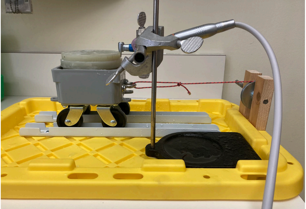
Figure 3. Standardized Force Generation Apparatus. The simulated dentin substrate (NEMA G-10) is affixed to a movable element on wheels, which is attached to a 100 g cylinder. The handpiece with bur inserted is affixed to a stationary element such that the bur exerts consistent force against the dentin substrate.
