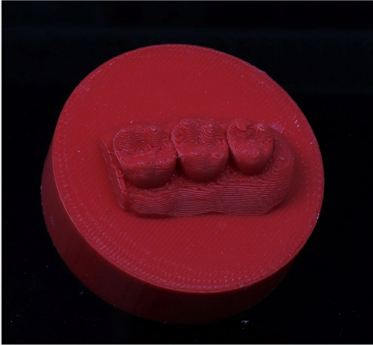
Figure 3. Image of 3D-printed custom sample holder. 3D-printed custom sample holder fabricated from a scan of typodont teeth #14, 15, and 16, designed on exocad software.
