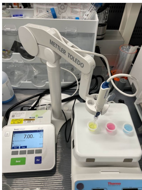
Figure 4. Calibrating the pH meter.
