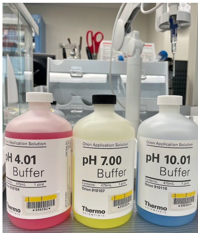
Figure 3. Buffer solutions used to calibrate pH meter.
