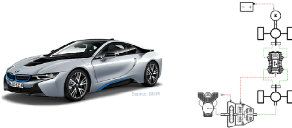
Figure 6: An illustration of the hybrid-electric powertrain of the reference BMW i8 vehicle
