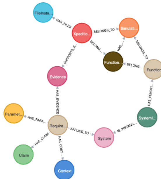
Figure 66: Domain Model of the KG Constructed using the Extracted Information
