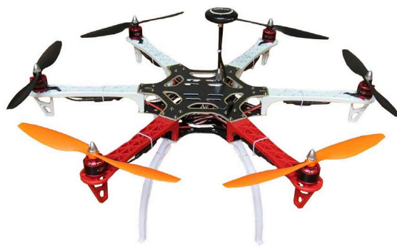
Figure 63: Hexacopter Design. The design space includes the choice of rotors, motors, batteries, and other components. These choices are discrete. Continuous design variables include e.g. the length of the arms and the pitch of the rotors. To find an optimal design, discrete and continuous variables must be optimized simultaneously. This is a mixed-variable high-dimensional optimization problem.
