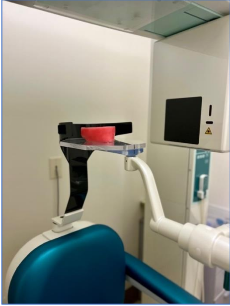
Figure 3: Samples on platform for scanning on 3D Accuitomo 80.
