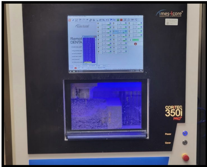
Figure 5: 350i 5 axis mill custom dry milling the bars
