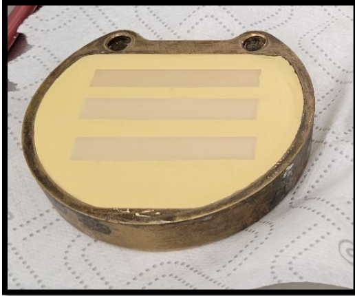
Figure 9.1 and 9.2: Wax bars fully seated in type 3 stone. Fully flasks PMMA in stone
