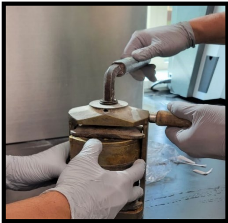
Figure 13.1 and 13.2: Closing of flask system. Deflasked PMMA
