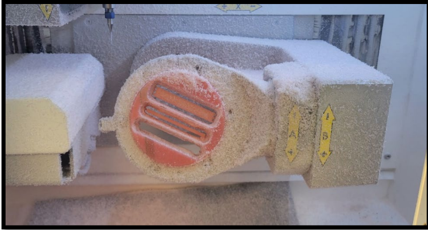
Figure 6: Finished bars immediately following milling
