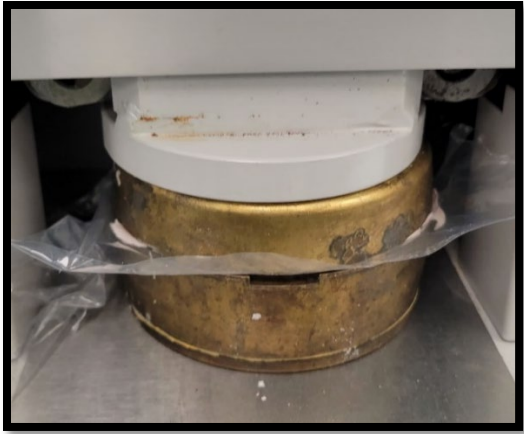
Figure 12.1 and 12.2: Condensing of PMMA. Nevin 832 Denture Flask Press
