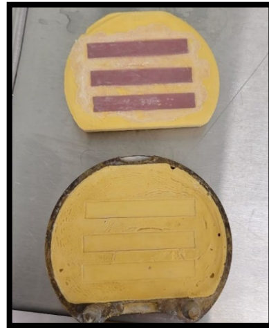
Figure 13.1 and 13.2: Closing of flask system. Deflasked PMMA
