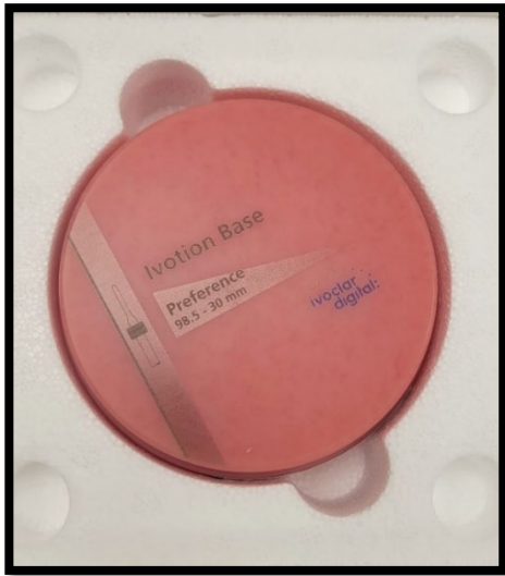
Figure 4: 98.5 x 30 mm Ivotion Base puck ready to be milled
