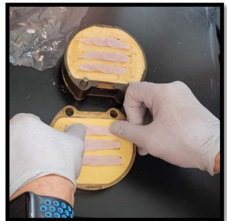
Figure 11.1 and 11.2: Mixing of Lucitone 199. Hand packing of PMMA.
