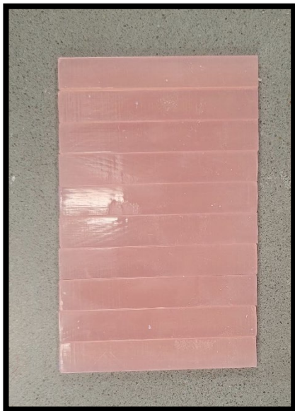
Figure 3: Denture base LP ready for testing
