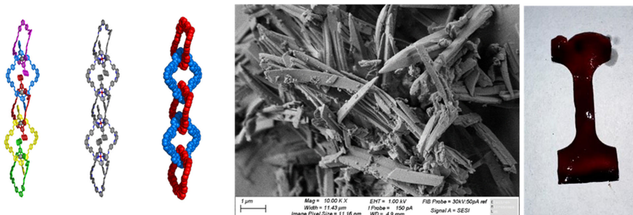
Figure 14. Poly(n)catenane COF. The proposed structure for the interlocked COF suggests the stacking of long 1D polycatenane chains. SEM micrographs of the samples show micron-sized crystals that can be used to generate a polycatenane film.
