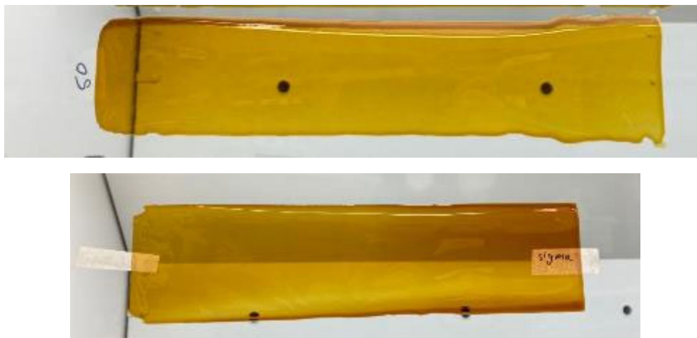
Figure 23. GRC synthesized polyimide (PI) film (top). Sigma-Aldrich (PYRE-ML) PI film (bottom).
