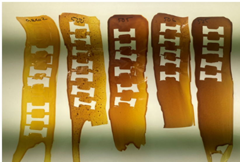
Figure 22. (left-to-right) GE Research Global Research Center (GRC) polyimide control, polymer composites with COF 500, 505, 506, 525.
