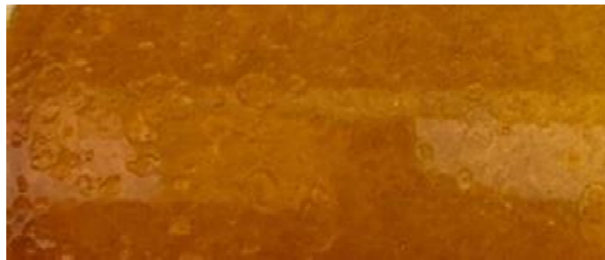
Figure 29. Polyimide film prepared from GRC F2701-95 polyimide.
