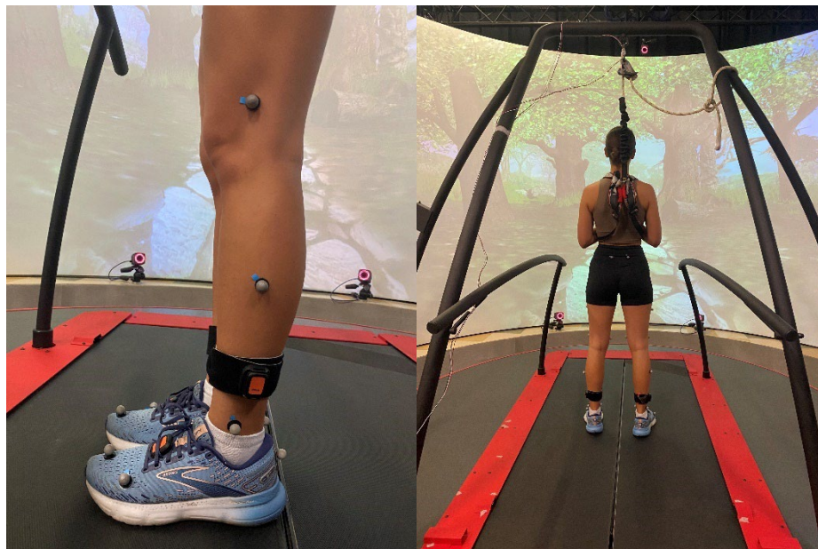
Figure 1. Image showing placement of the IMU sensors on the lower limb region (left) and the set-up with reflective markers on the motion base treadmill (right).
