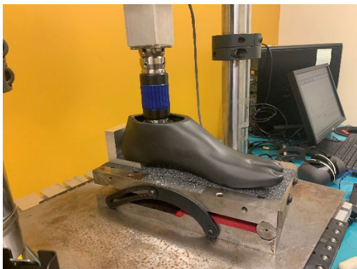
Figure 1: the research team at Northwestern University/Jesse Brown VA Medical Center has previously validated a bench testing method to quantify mechanical characteristics of prosthetic components (e.g., stiffness, energy return or dissipation), representative of unique loading patterns encountered during different phases of walking (e.g., early stance, midstance, and terminal stance). In this project, the bench testing method was applied to quantify the properties of two different prosthetic foot/ankle components, with and without shock-absorbing pylons of varying levels of hardness (see Figure 2).
