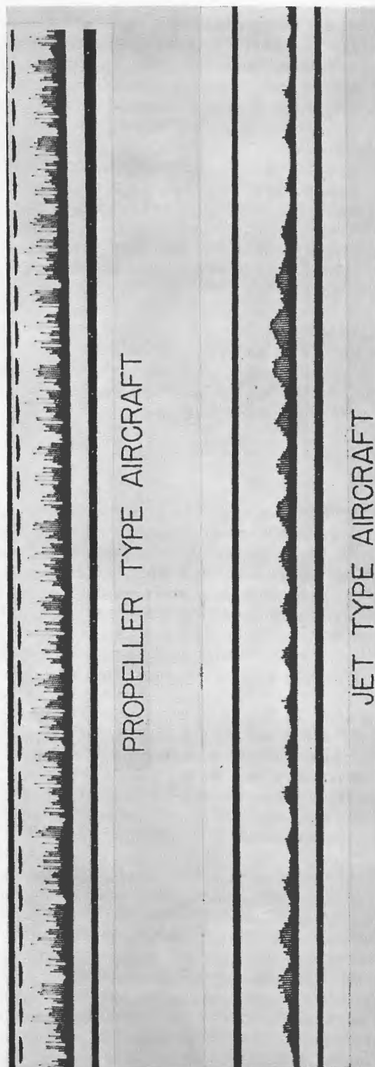
Fig. 1 - Pulse-by-pulse recordings of fire-control radar echoes
