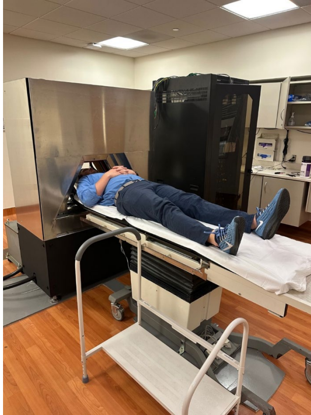
Figure 1. Stationary head CT components in the former clinical CT space at the UNC Hospital's Ambulatory Care Center. The x-ray tubes and detector assembly are contained within the stainless steel shell. The subject is positioned near the end-scan phase of the imaging. A step stool is provided to assist subjects.
