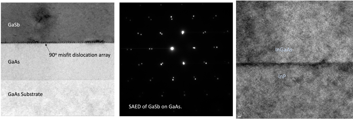
(a) (b) (c) Fig. 6. TEM analysis of IMF formation between the GaSb/GaAs layers. Figure (a) shows all three layers, (b) is an SAED analysis of figure (a). (c) shows the growth interface between InGaAs on InP.
