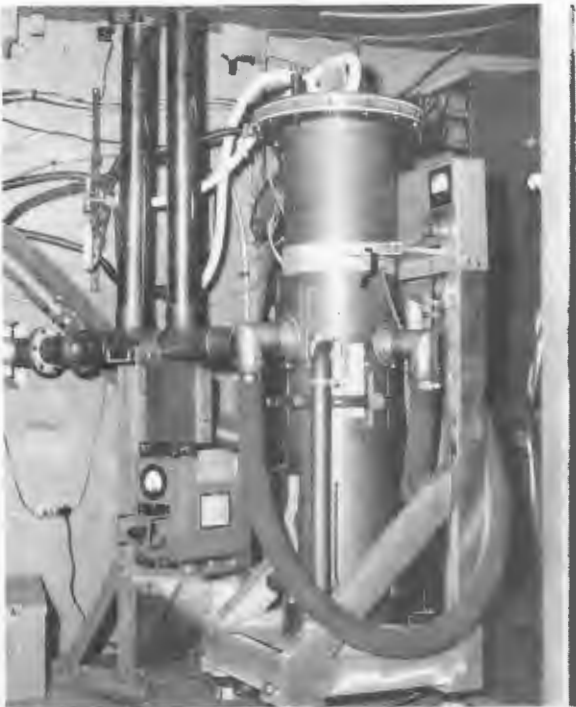
(c) Transmitter assembly with tuning stubs and type OA-2 frequency meter
