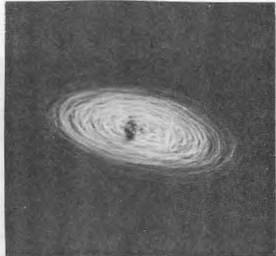
Fig. 43 - Indicator display of signal radiated by local power lines, taken November 26, 1954. Frequency, 8.5 kc, true bearing, 106 degrees.
