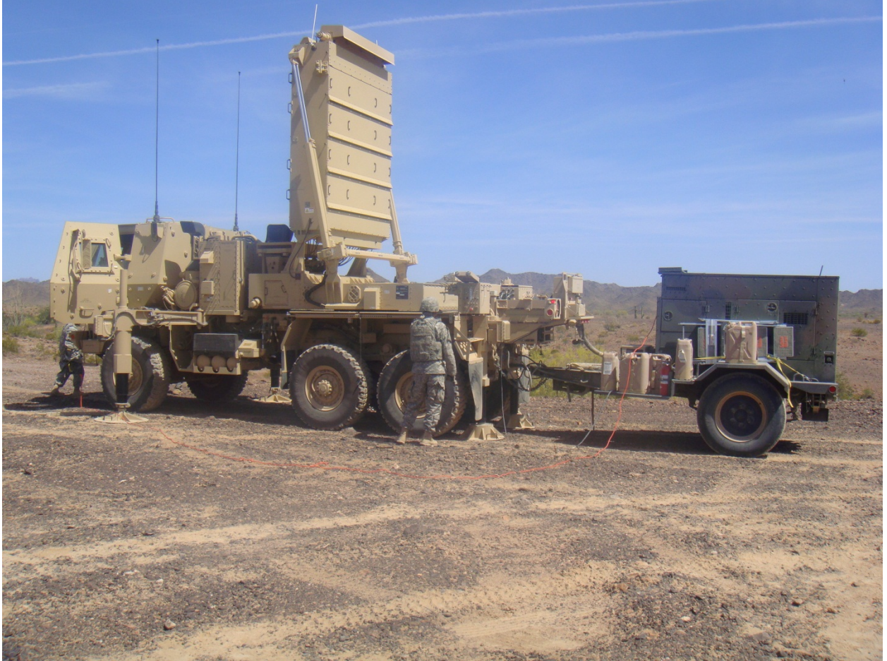
Figure X.14 – Soldiers emplacing the Q-53 radar during operational testing.
