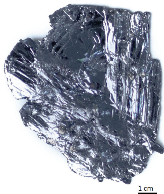
Figure 1.4: \text{MoS}_2 in its bulk form. From this flake, multiple samples can be mechanically exfoliated. This piece and every piece like it are made up of millions of individual layers of variable size. Figure reproduced from Spi supplies [11]
