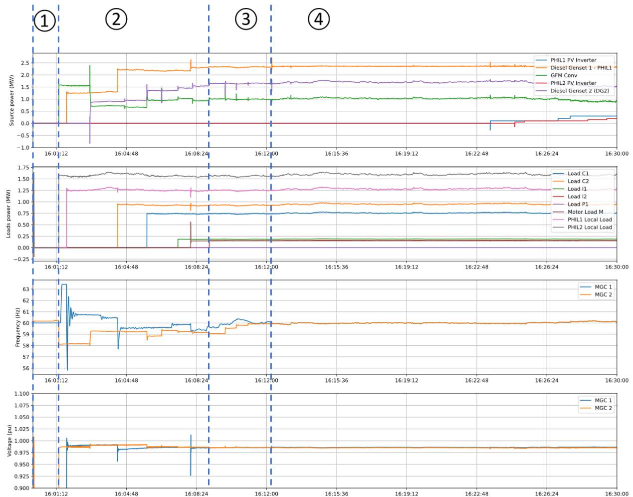
Figure 6-3. Black Start Process with 4pm Profile N Strategy
