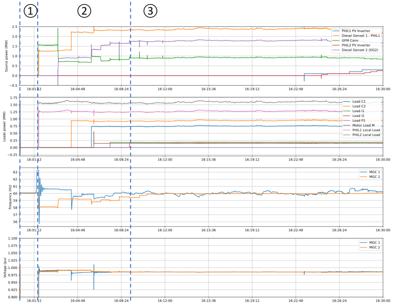
Figure 6-5. Blackstart Process with 4pm Profile Separated Microgrids
