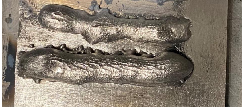
Figure 9 Single and double layer bead of magnesium using synergic pulse welding
