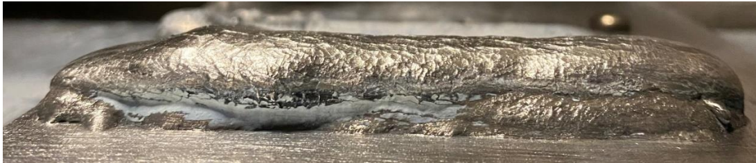
Figure 10 Side view of double layer bead of magnesium using synergic pulse welding
