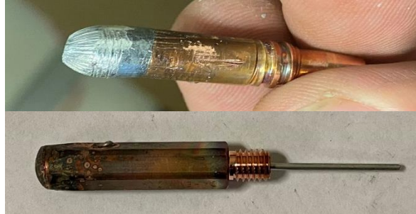
Figure 6 Melted contact tips from Mg GMAW
