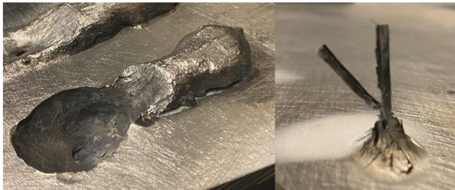
Figure 7 Burn through of magnesium substrate
