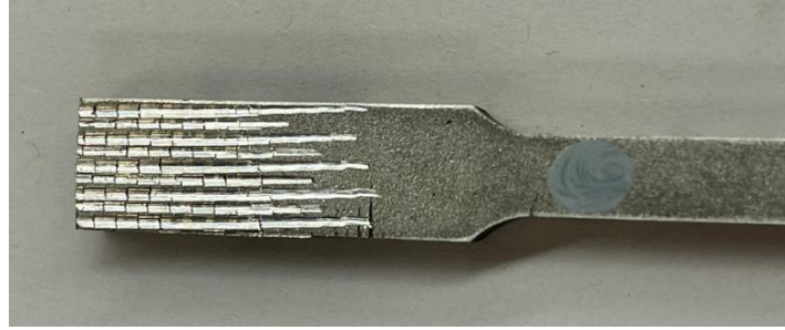
Figure 29 Specimen slip and deformation during tensile test
