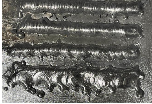
Figure 16 Side flow of overlapping beads
