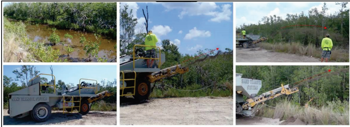
Figure 8. Sand transfer system (sand shooter) used to place sediment in a 2012 mangrove mitigation enhancement project in Miami-Dade County (photos credit: Miami-Dade County, Florida).
