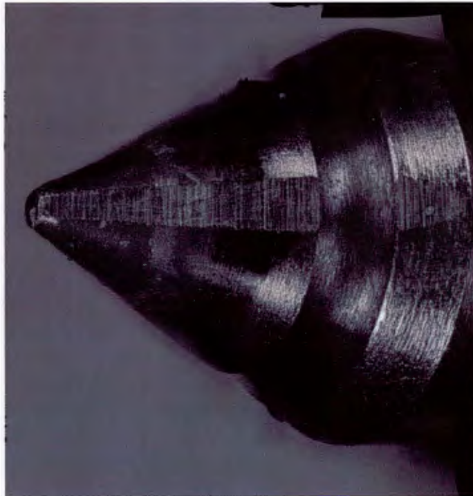
Figure 8 – Precision ground flat spots on the side of the injector valve nozzle
