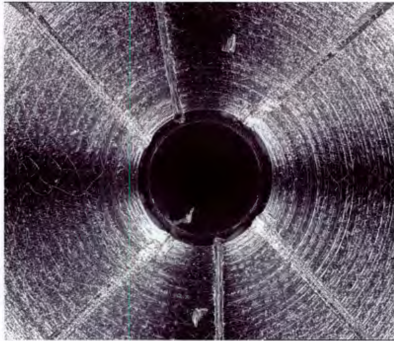
Figure 7 - Scratches in the solenoid valve ball seat allowing leakage
