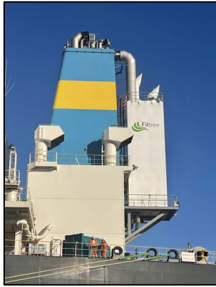
Figure 23. Carbon Capture System on EPS-Managed Tanker (EPS)
