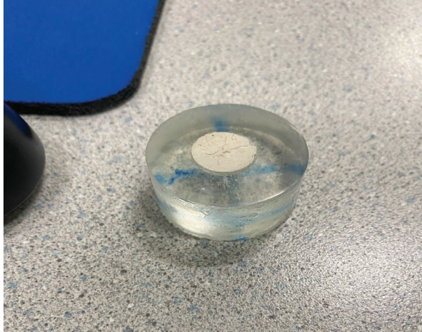
Figure 7. Image of a sintered sample after mounting in an epoxy. The corner of a standard mouse pad is seen for reference.
