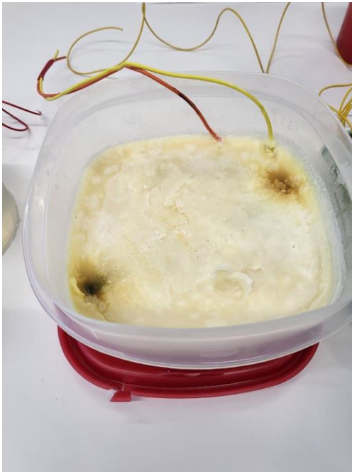
Past ultrasound phantom prototype investigating the use of cocoa butter/palm oil mixture.
