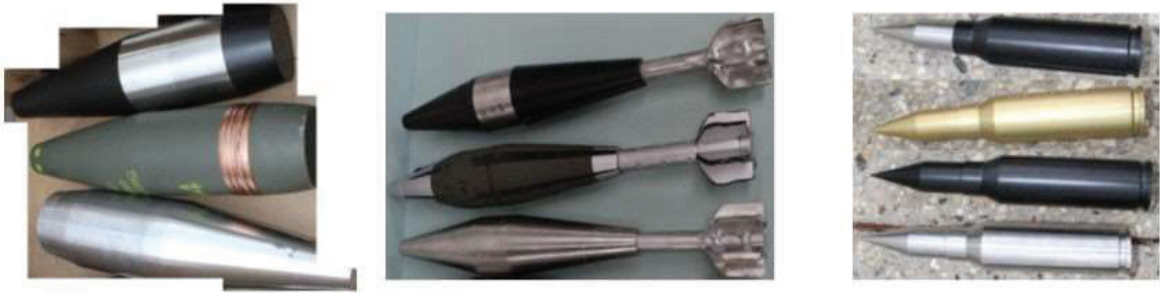
Figure 1. Fabricated surrogate, purchased replica, and fabricated replica of (left) 155 mm HE M107, (middle) 81 mm mortar, and (right) 25mm and 20 mm cartridges (from Calantoni et al. 2014).
