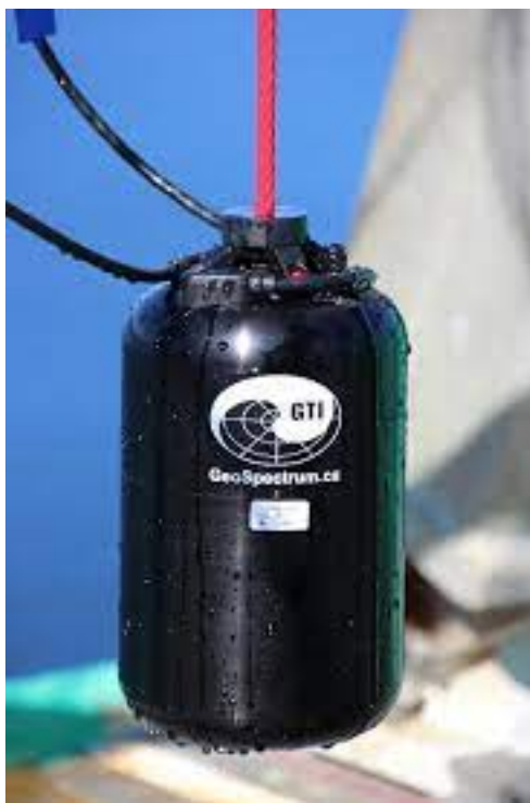
Figure 2.3. Geospectrum M20-105 Vector Sensor. Source: [18]. A single vector sensor can measure the pressure and direction of a sound wave using pressure sensor and particle motion sensors. The Geospectrum M20-105 vector sensor can detect a frequency range of 1 Hz to 3,000 Hz. Thus, it is capable of detecting marine mammals, particularly blue whales as the frequency of their calls is between 10 Hz to 100 Hz.
