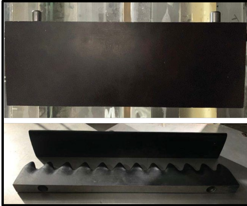
Figure 18. a) Airfoil body and b) interchangeable leading-edge
