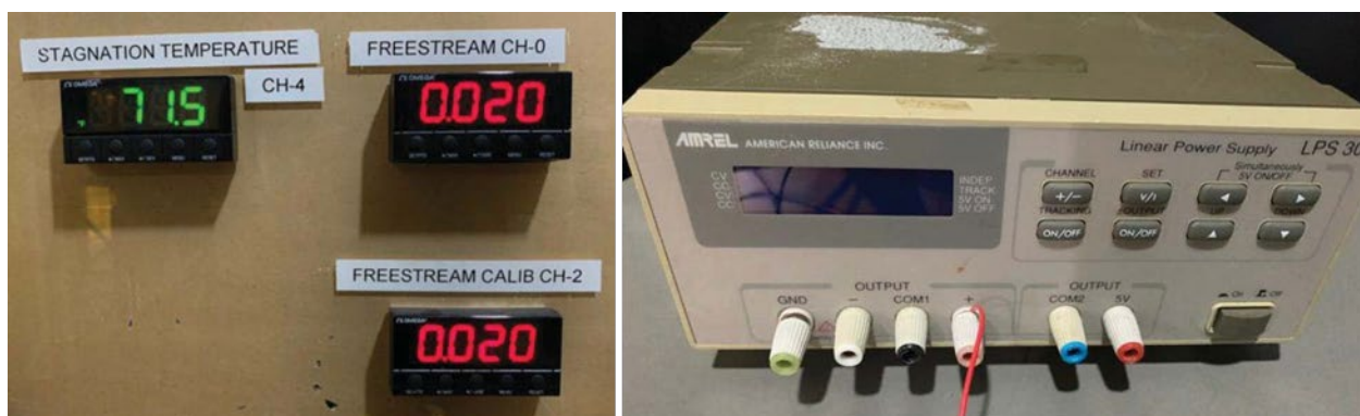
Figure 28. a) Display of test section conditions and b) linear power supply (LPS) 304
