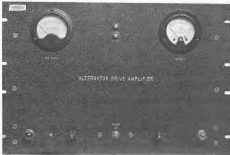
Fig. 7 - Panel view of the power amplifier
