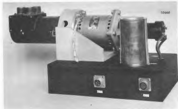
Fig. 13 - Goniometer and alternator connected to the synchronous drive motor
