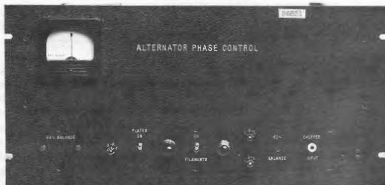
Fig. 5 - Panel view of the alternator phase control chassis
