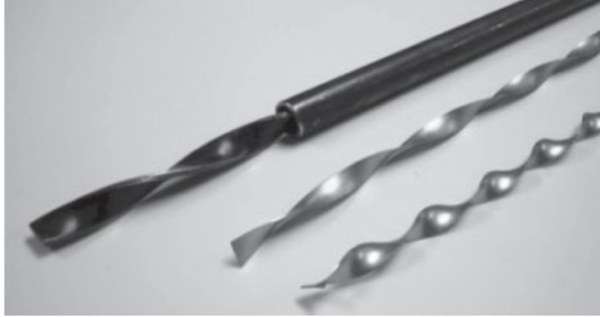
Figure 6. Several examples of twisted tape inserts. Source: [5].
