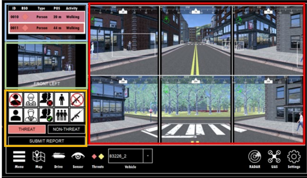
Fig. 1 Target classification task interface (right-hand monitor). Windows are (clockwise from right) indirect camera vision feeds (red border), agent reasoning and transparency (yellow border), snapshot of selected person (green border), and list of identified persons (blue border). For additional details see Section 3.4.
