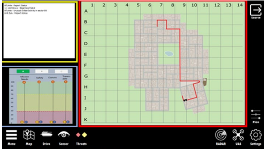
Fig. 2 Environment awareness interface (left-hand monitor). Windows are (clockwise from right) top-down map of the area showing vehicle and its route (red border), route selection logic (blue border), and command chat window (yellow border). For additional details see Section 3.4.
