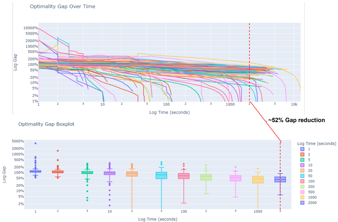
Figure 4.9. This figure depicts two plots illustrating the optimality gap over time for the mean lateness objective. The axes of the plots have been logarithmically scaled to condense the represented values. The x-axes represent time in seconds, while the y-axes represent gap as a percentage. The upper plot shows the optimality gap over time for each scenario, while the lower plot displays the five-number summary (minimum, first quartile, median, third quartile, maximum) for all scenarios at those time intervals.
